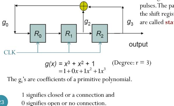
alphabet  $\{0,1\}$  are shifted through the shift register in response to clock pulses. The particular 1s and 0s occupying the shift register stages after a clock pulse
